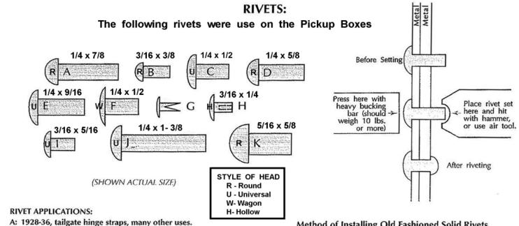
B: 1926-31, fender spacers, bed strips. C: 1926-52, bed assembly, 1926-31, tailgate hinges, many other uses.
